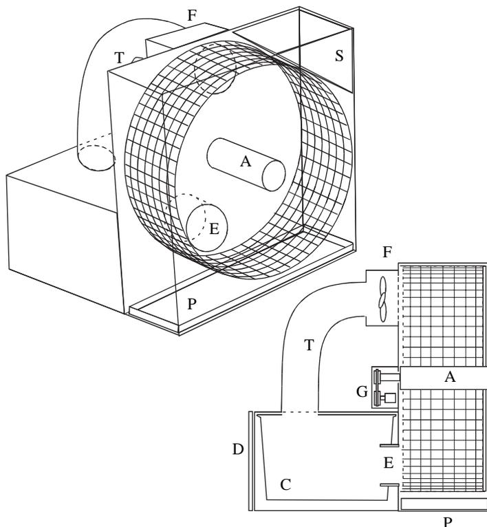
Fig. 1. Schematic diagram of the running wheel enclosure. A, wheel axle (attached to the back side of the housing); F, fan; T, recirculation tube; C, mouse cage; D, access door; E, wheel entry tube; P, waste pan; G, wheel speed generator; S, space filler. Not shown: food hopper, drinking tube, air access ports, other space fillers in corners of wheel housing and around mouse cage. The internal volume (without cage, bedding, and food) is approximately 22.7 liters.
